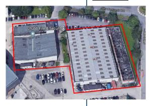
Demolition of 2No large portal frame structures; one single storey and one part three-storey; 44,000ft2 in total plan area.
